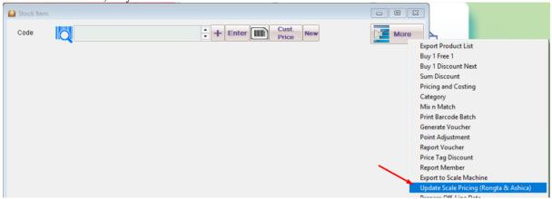
Key in ip address of scale machine, and click Scale Icon.
